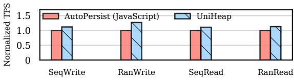
Figure 9: Performance of SpiderMonkey in UNIHEAP. data accesses to persistent objects in UNIHEAP can scale to support multiple managed runtimes.
